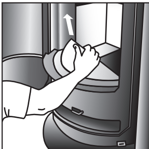
Changing the firebricks/vermiculite plates (begin with the stone at the front)
